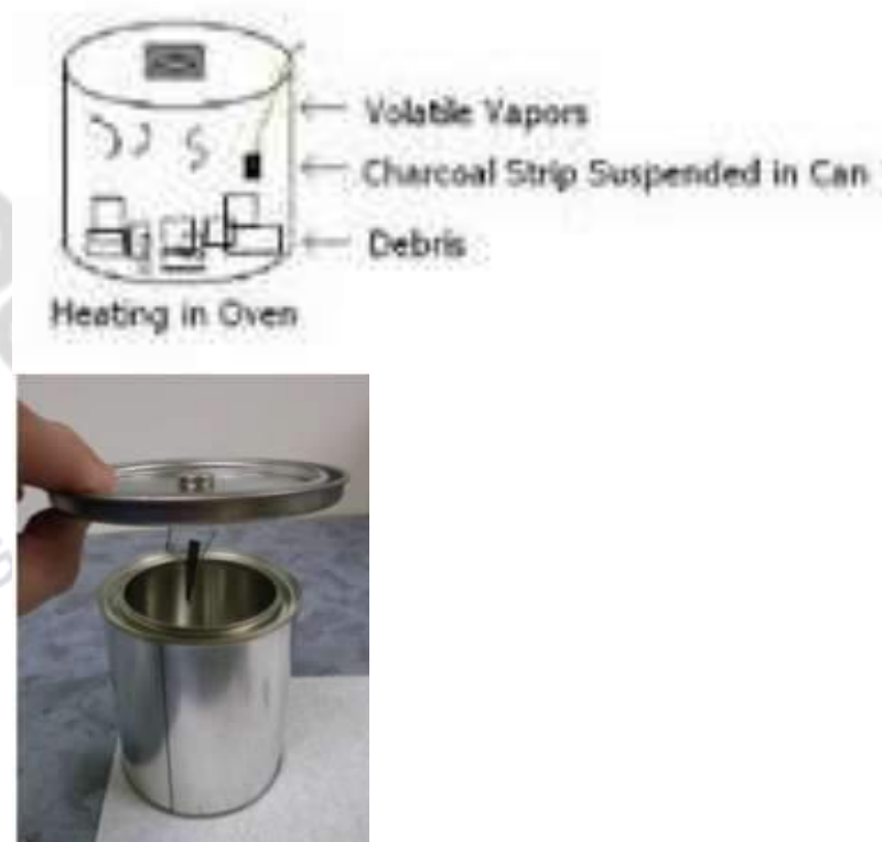
Figure 7: Vapour concentration using charcoal strip
